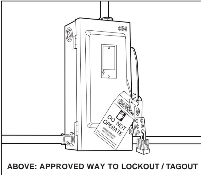
The energy isolating device must bear a prominent warning tag indicating that work is being done on the equipment and the name of the authorized employee responsible for the lockout. It is mandatory that tagout notices not be susceptible to deterioration or illegibility due to weather conditions or exposure to chemicals and moisture.
