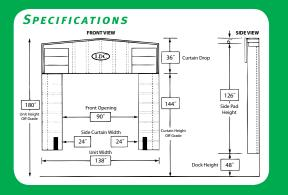
Generally designed for but not limited to 10' wide x 10' high openings. The series D600 is ideal for tailgate or standard trailers. The design of this unit allows the trailer to pass through the side and top curtains allowing full unrestricted access to the rear of the trailer when loading and unloading.
